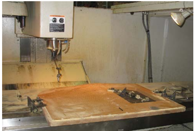
Figure 11. Composite Door Fabrication
