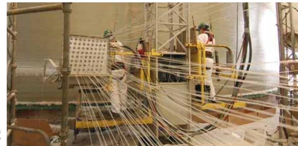
Ershigs (U.S.) has produced filament wound FRP vessels that are 88 feet in diameter and 75 feet high (26.8 x 22.9 meters).
