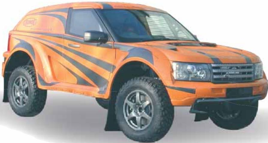
Twintex reinforcements are delivering their special performance properties in another challenging application – bodies for cars used in off-road racing.
