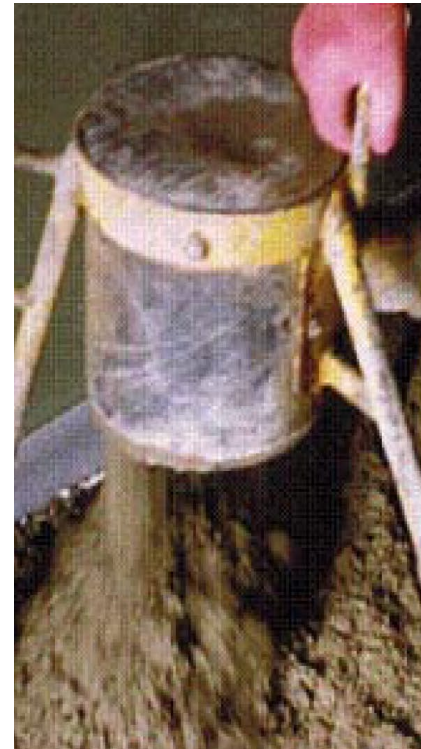
The mix is perfectly workable, easy to be pumped and leveled. No fiber on surface
