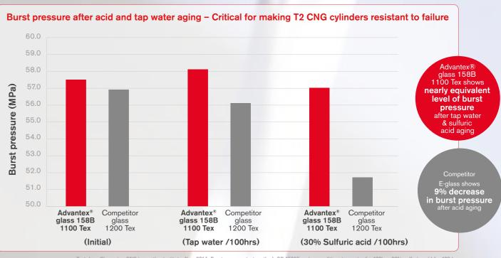
Test done Chongging CNG inspection institute, Nov. 2014. Burst pressure test method: GB 15385; aging condition: tap water for 100hrs, 30% sulfuric acid for 100 hrs.
