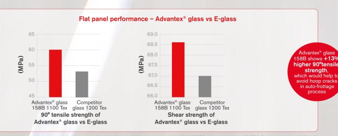
Test done Chongqing CNG inspection institute, Nov. 2014. 0°/90° Tensile strength method: ISO 527-5; Shear strength method: ISO 14130.
