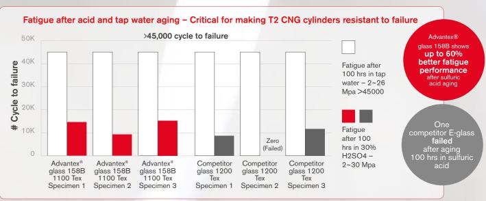
Test done Chongqing CNG inspection institute, Nov. 2014. Fatigue test method follows GB 14260.
