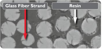
Scanning electron pictures are from Owens Corning corrosion lab in 2011.
