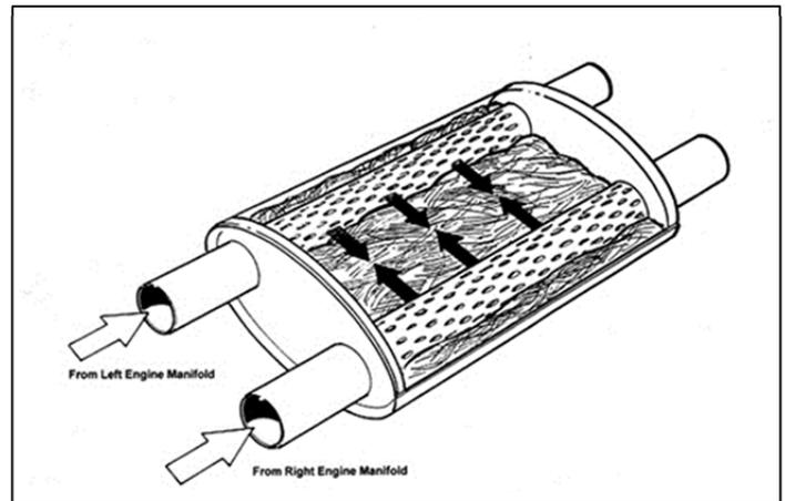
Figure 7: Particulate blowout from gas flow through the roving.
