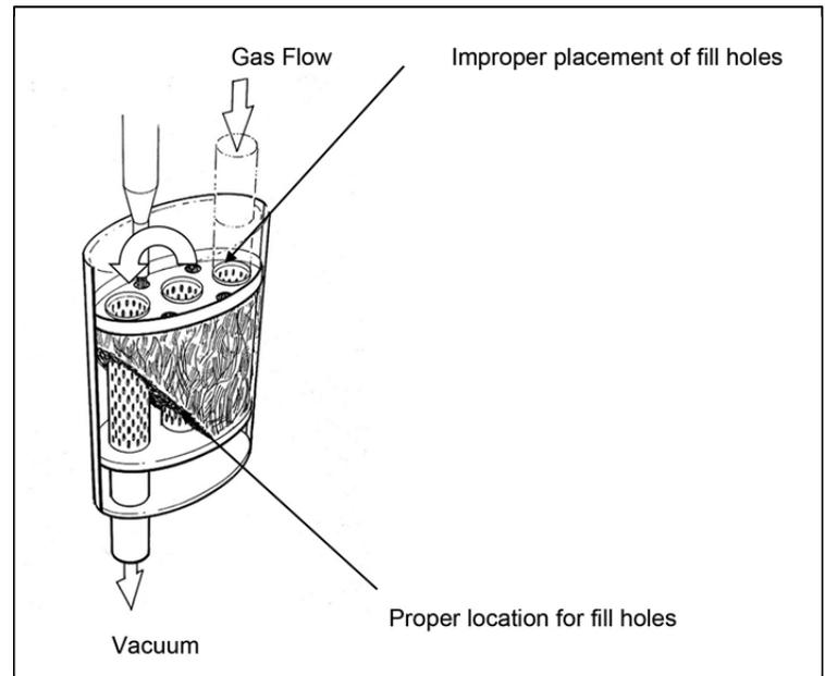
Figure 5: Placement of fill holes for direct fill of round and oval silencers.
