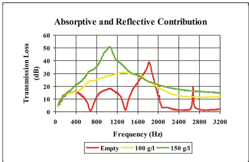
**Figure 1:** Acoustic transmission loss of a simple expansion chamber approximately 16 cm. in diameter and 25 cm. long containing a 5 cm diameter perforated tube with 8% porosity.
